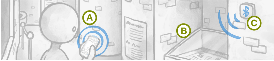
Fig. 1. Museum setting showing the visitor using the mobile application with visualization (a), the physical object in the museum (b), and Bluetooth beacons at exhibits telling the app where the user is located (c).
