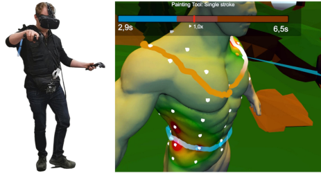
Fig. 12. VRTactileDraw driving a 52-actuator tactile vest mockup, and the users’ view inside an HTC Vive
