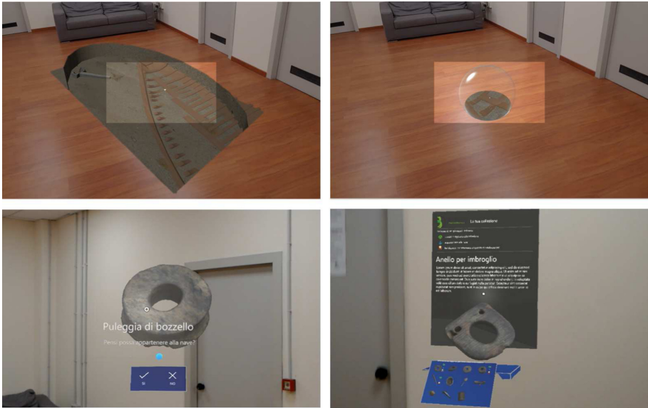
Fig. 1. (left to right, top to bottom) Used HMD's narrow FOV able to shows only a portion of the scene which for this reason was hidden under the physical floor; the sphere widget, fully visible in the FOV of the device, that collides the floor opening a breach over the archaeological excavations; manipulation of the collected finding, the text shows the finding name Puleggia di bozzello and the question Do you think it could belong to the ship? ; interactive panels for the presentation of cultural information related to the artifacts collected.
