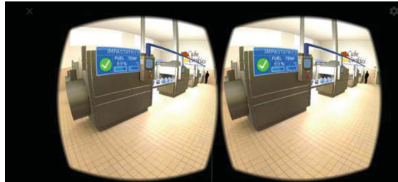
Fig. 2. Production units with annotations in the Cube Cookies Factory. Navigation and interaction are performed with cardboard, through a smartphone.
