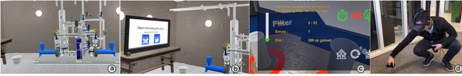
Fig. 1. Overview of VRQUEST system (a) 1:1 scale 3D model of the cooling system (b) a virtual screen allowing the user to choose the training mode ( Tutorial or Practice ) and view the instructions in Tutorial mode (c) summary of user performance when completing the task in Practice mode (d) a participant bending down and reaching his hand over a virtual pipe to turn a valve located close to the floor.
