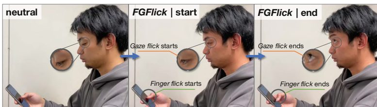
Fig. 1. FGFlick overview. The user flicks with a finger on a smartphone while he also moves his gaze linearly.
