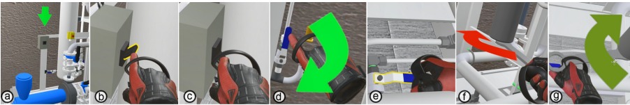
Fig. 2. Examples of user interactions in VRQUEST . (a) An arrow helps the user locate a switch (b) the user's virtual hand forming a pointing gesture with the index finger placed on the switch (c) then flicks down to turn it off (d) an arrow indicating the location and the rotation direction of a valve (e) grabbing the valve handle to rotate it (f) removing the nut of the filter using a wrench, the arrow indicates the rotation direction (g) the user turning the wrench in the indicated direction.
