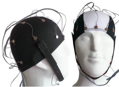
Fig. 3. HapticHead for vibrotactile feedback around the head [26].
