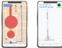
Fig. 1. An example of the front end design of the application: the red areas are indicative of the presence of crowded roads. The navigation systems determines an alternative route to reach the destination based on the objective of minimizing the potential exposure to crowded places.
