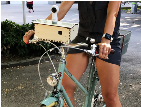
Fig. 1. The hardware iteration of the Virtual Cycling Coach used in the second evaluation round: Mounted on the handlebar, the casing housed a front-facing camera that live-streamed a video feed to the controlling researcher (the wizard), a smartphone with an attached loudspeaker for outputs of the audio interface, and a 360° camera on top for recording the session.
