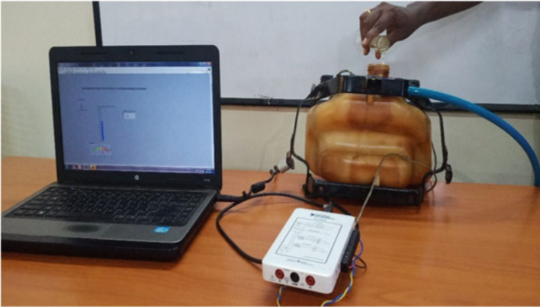
Fig. 13.2 Experimental setup of the volume measurement system
