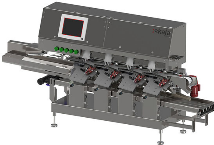
Fig. 19.1 Fully automated vaccination machine used in large-scale salmon smolt farms. https://www.skalamaskon.no/aquakultur/vaksinering
