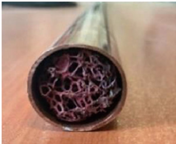
Fig. 8 Porous structure used in the experimental setup of novel and rival Flat plate collector. Reprinted from Ameri et al. (2018)
