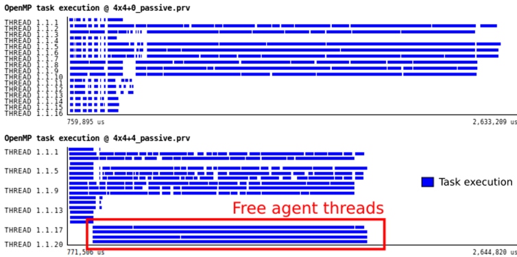
Fig. 1. DMRG++ trace execution with a 4,4 nesting running on 16 CPUs, and same execution running with free agent threads. Both traces are at the same duration time scale.
