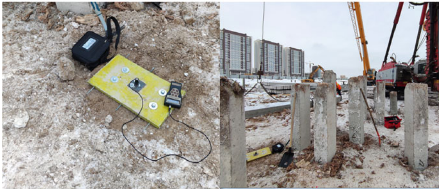
Fig. 2 Installation of vibration monitoring sensors
