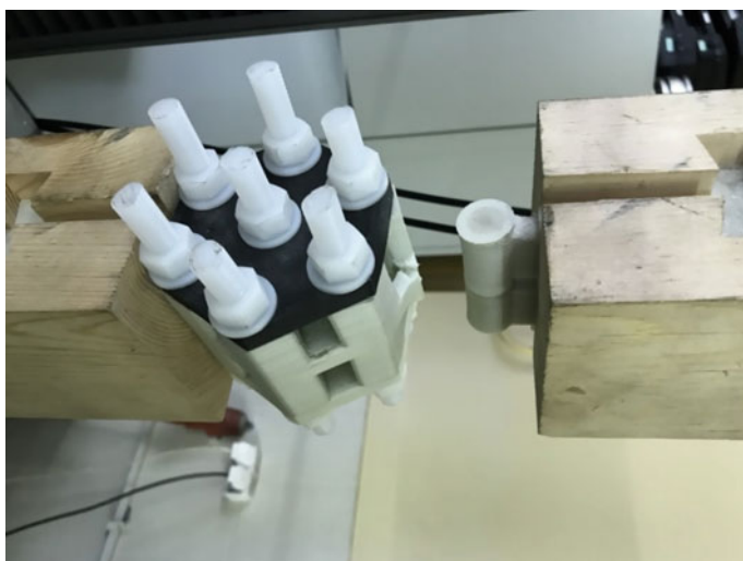
Fig. 8 The destroyed node
