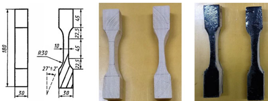
Fig. 2 Tensile test piece at an angle to the fibers
