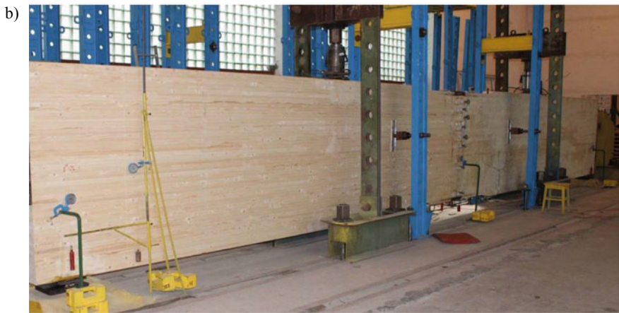
Fig. 6 Scheme and general view of testing the specimen joint. LWB1 and LWB2 – glued laminated timber elements; a hydraulic jacks DG100; b steel frames anchored in the load-bearing floor
