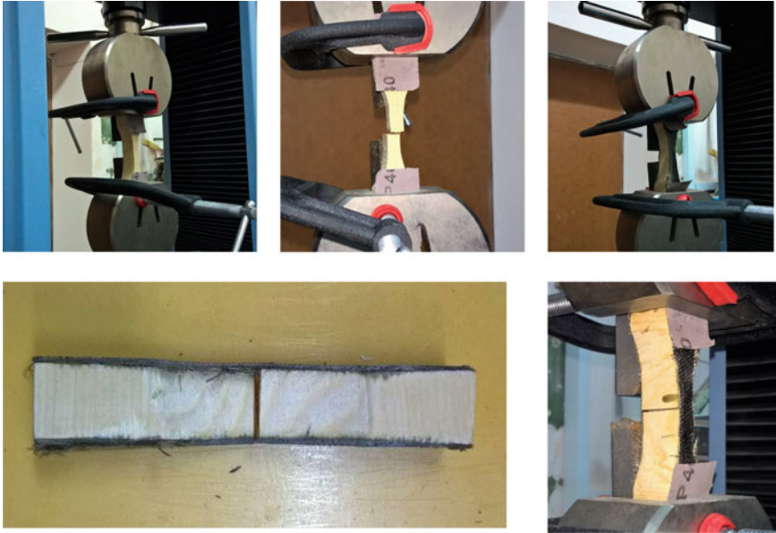
Fig. 3 General view of the test and tested prototypes in tension at an angle to the fibers
