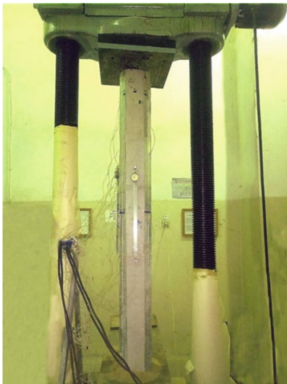
Fig. 10 Test stand with testing steel–concrete column
