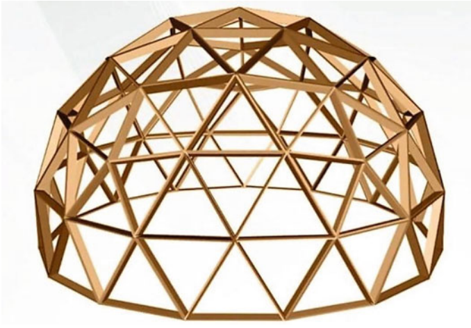
Fig. 3 The frame of the building in the form of a geodesic dome
