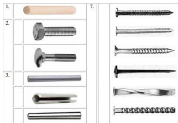
Fig. 1 The main types of dowels used in the joints of wood structures (1 oak dowel, 2 bolts, 3 pins, 4 screws, 5 self-tapping screws, 6 ordinary screws, 7 nails)
