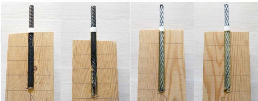
Fig. 3 Samples tested by the pull- out test. Rectilinear trajectory. Reinforcing deformed steel bar and steel wire rope
