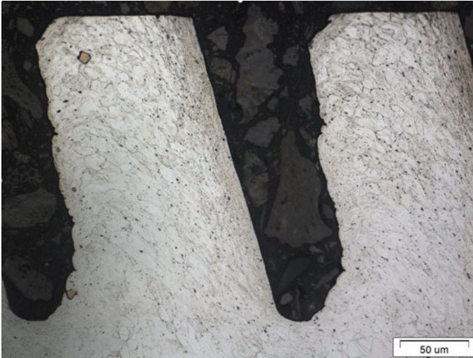
Fig. 5 Microstructure of the fin material of AISI 321 steel, \times 500
