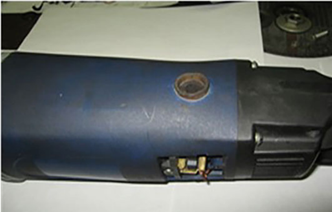
Fig. 9 Test bench with a window for grinding composite
