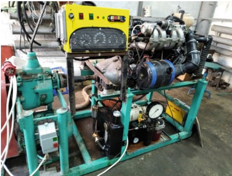
Fig. 2 Stand with the ability to provide loading modes by instrumental methods and an electric motor in its design
