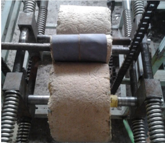
Fig. 1 Test bench for moisture squeezing out of semifinished leather products
