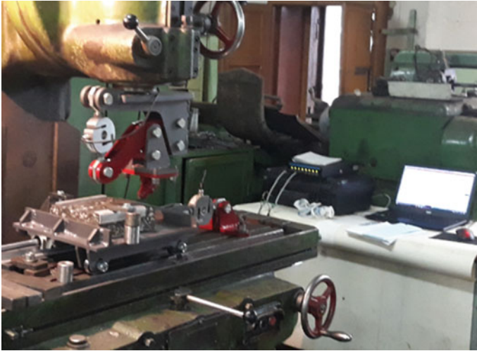
Fig. 2 Experimental bench to study asphalt concrete cutting with a single cutting element of a road milling machine
