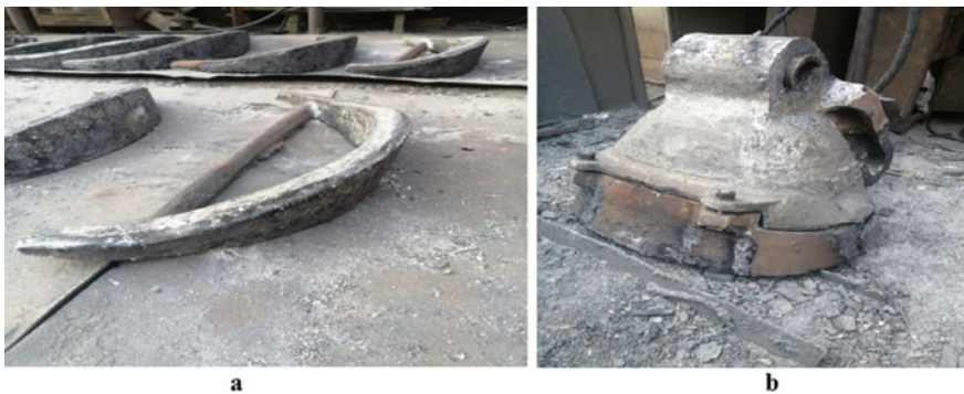
Fig. 4 a Visor used to restore the scoop; b dredge scoop (250 l) restored by welding
