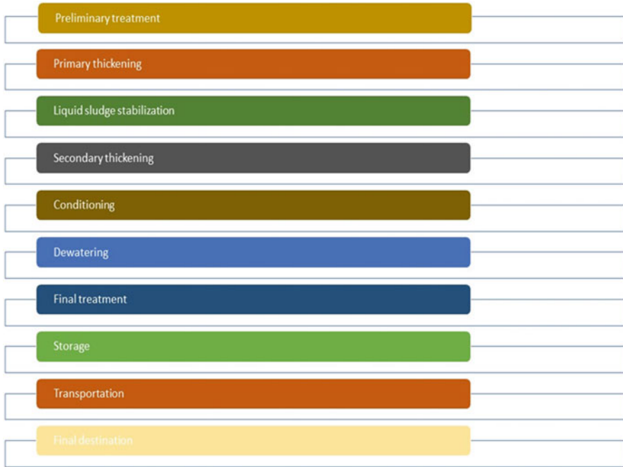
Fig. 1 The different step which generally uses to process sewage sludge to using it as fertilizer
