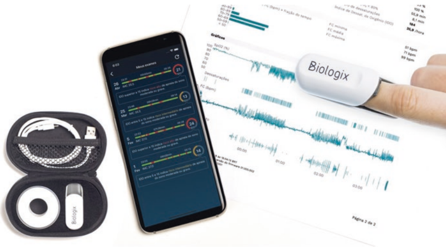
Fig. 3 Wireless pulse oximeter coupled with an internal accelerometer, destined to remotely monitor the risk patients. (Reprinted with permission from Biologix)
