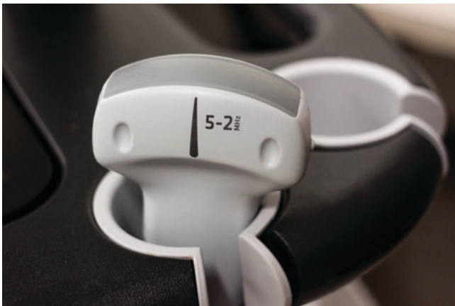
Fig. 78.2 Curved array transducer with a larger footprint and better resolution for deeper imaging that can be used for FAST examination as well as lung examination
