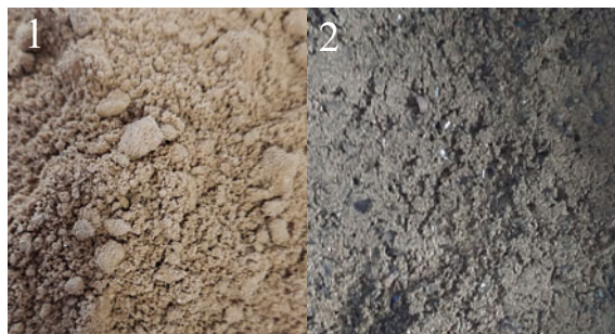
Fig. 1 General view of the components of the mixture: 1—loam loess disturbed structure of natural humidity; 2—fly ash of the Mikolaev CHP
