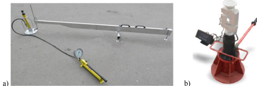
Fig. 1 Measuring equipment for static stamp tests: a NTU stamp equipment; b SNPTs «ROS-DORTECH» press-stamp PSH-050
