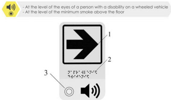
Fig. 20 Examples of a sound-signaling beacons combined with an information plate and a tactile resource book: 1–flatly printed graphic information, 2–duplication of flatly printed graphic information in Braille type, 3–play button for reproducing audio information
