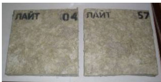
Fig. 1 Exterior view of the samples before (sample at the left of the Figure) and after (sample at the right of the Figure) 180 cycles of climate impacts
