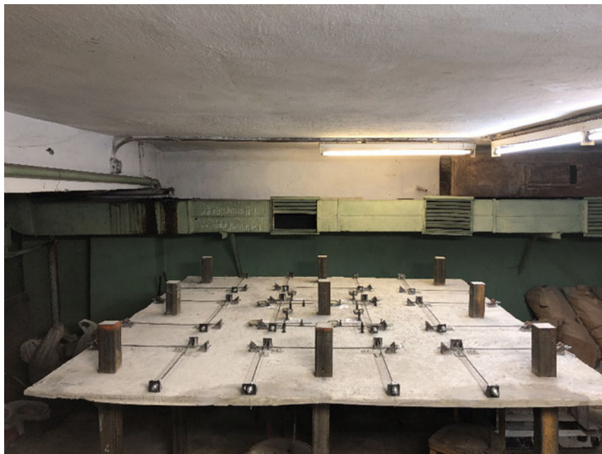
Fig. 2 Research model of reinforced flat slab
