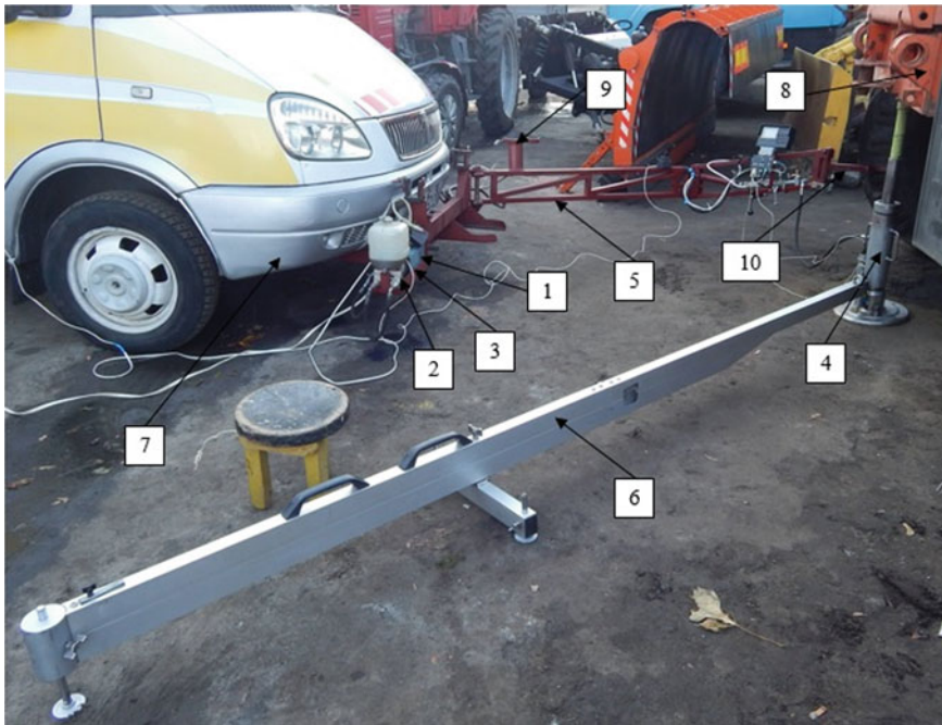
Fig. 3 General form of the measuring station mounted on the basic car “GAZelle” (photo Ivan Shuliak 2016) 1 – pumping station; 2 – hydraulic pump; 3 – engine; 4 – a stamp with the hydraulic cylinder; 5 – lever-holding mechanism; 6 – deflectometer; 7 – basic car; 8 – loading means; 9 – mounting bracket; 10 – grip of the lever-holding mechanism
