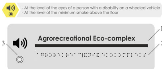
Fig. 19 Examples of an audio indicators combined with an information plate and a tactile resource book: 1–flatly printed textual information, 2–duplication of flatly printed textual information in Braille type, 3–play button for reproducing audio information
