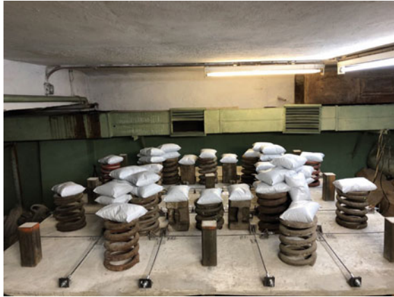
Fig. 6 Loading for experimental model. Second stage—sum loading 581 kg
