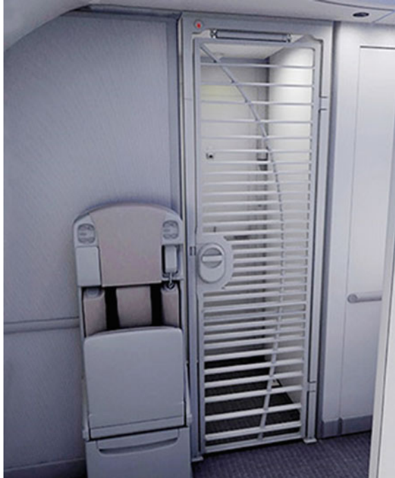
Fig. 4.1 Secondary Flight Deck Barrier (Installed Physical Secondary Barrier or IPSB) [14]
