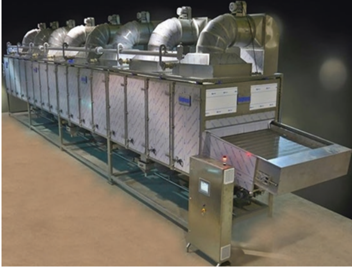
Fig. 1.3 Conveyor dryer. (Courtesy: Bigtem machines, Turkey)
