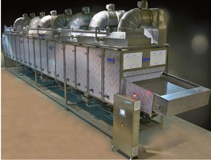
Fig. 1.3 Conveyor dryer. (Courtesy: Bigtem machines, Turkey)
