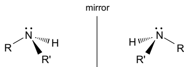
Fig. 15.1 Non-superimposable mirror image of an amine with four different groups around N
