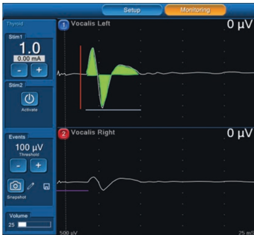
Fig. 11.2 Nerve integrity monitoring display with amplitude (red bar), duration (blue bar), phase (green), and latency (purple bar) of a typical EMG motor unit action potential
