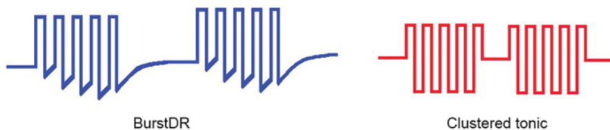
Fig. 4 Illustration comparing BurstDR stimulation with nonlinear charge accumulation and Burst stimulation modalities resembling a clustered tonic stimulation
