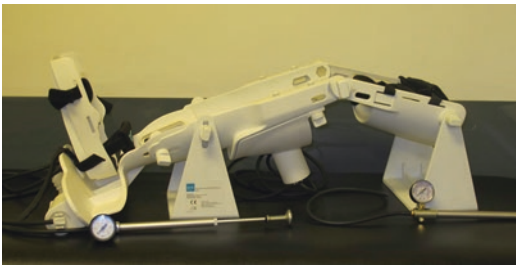
Fig. 8.1 Photograph of the Porto-Knee Testing Device (PKTD)
