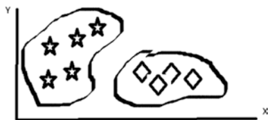
Fig. 4 DBSCAN clustering . DBSCAN clustering, as a density-based clustering algorithm, can classify data into any shape of clusters in a dataset. Sparse areas are borders between clusters that are required to separate clusters. Any data that lies in this area is considered to be a broader point corrupted by noise
