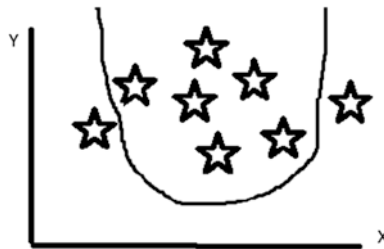
Fig. 9 Overfitting. In this example, overfitting is created by using a quadratic function that fits too well on the training data and noise. There are few samples that are not covered in the quadratic function. Thus the model does not categorize the data correctly because of too many details and noise
