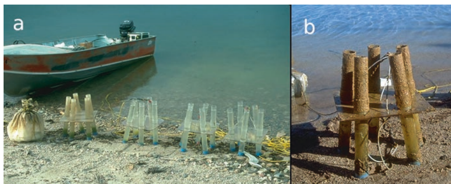
Fig. 9.1 Sediment traps used to collect and analyze particulates. (a) The traps on the left were installed at depths between 3 and 45 m. The traps closest to the boat had a fine layer of clay which was not visible on any of the following traps. (b) Photograph of the 3 m depth traps one year after flooding, showing the high quantity of suspended solids (Boojum Research, 1994; Cao & Kalin, 1999; Kalin et al., 2001). (Photographs by Boojum Research)
