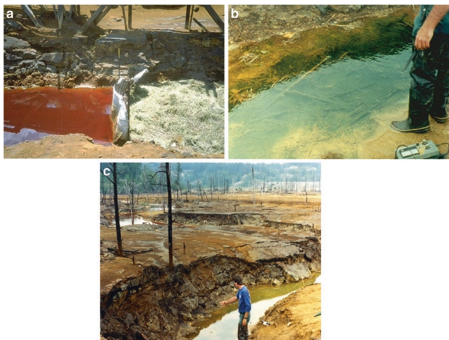
Fig. 4.4 (a) Pyrrhotite tailings crust. In the foreground is the creek in which the first straw addition was made. (b) Straw addition in acidic creek before winter at the time of setup. (c) Clear section of creek with straw in spring, all iron had been precipitated. (Photographs by Boojum Research)
