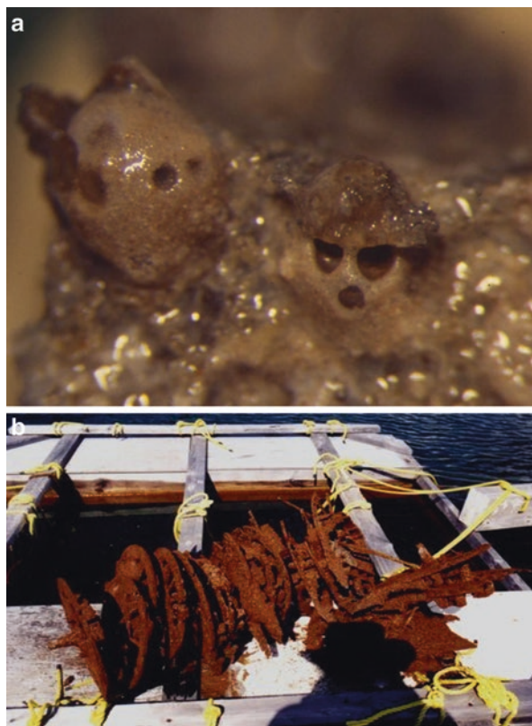
Fig. 7.11 (a) A close-up photograph of corrosion channels with hydrogen bubbles, due to continued corrosion. (b) Magnesium scrap metal on a string covered with iron and magnesium after being suspended from a barge in an acid lake. (Photographs by Boojum Research)
