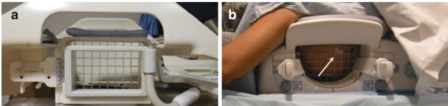
Fig. 10.32 (a) Breast coil and biopsy grid from Siemens (a) and from General Electric (b). The fiducial marker is placed in one of the grid holes (arrow) to serve as a landmark for hole identification on MR images
