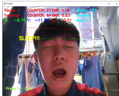
Fig. 9. The detection of a fatigue driving behavior
