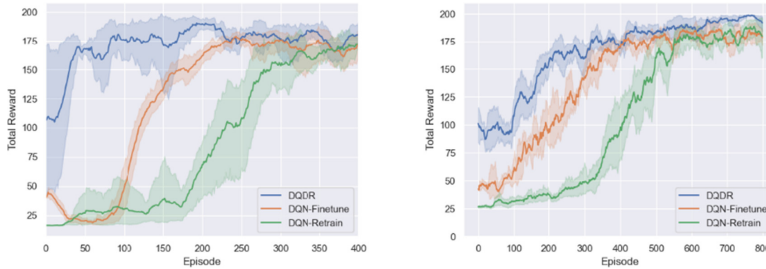
Fig. 6. Experimental results of the pole length transfer (left figure) and cart weight transfer (right figure) on CartPole task. The shaded region denotes the standard deviation of average evaluation over 5 trials.
