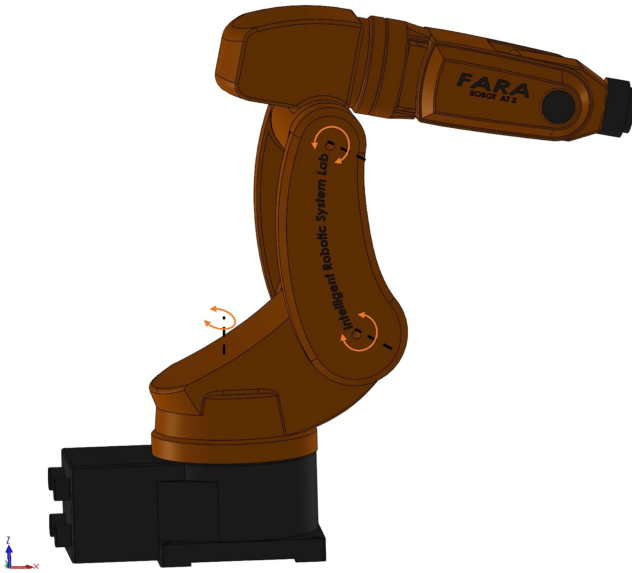
Fig. 3. 3D SOLIDWORK model of the 3-DOF FARA Robot Manipulator
