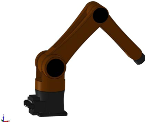
Fig. 1. 3D sketch of a 3-DOF manipulator with SolidWorks.
