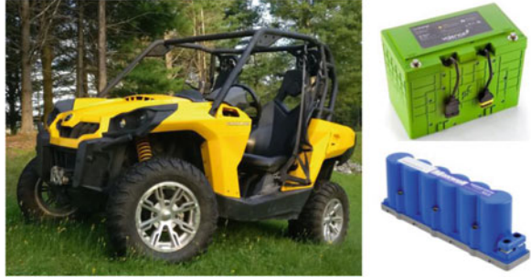
Fig. 7 The eCommander EV with the associated Valence U24-12XP Li-ion battery and Maxwell BMOD0058 E016 B02 SC modules of e-TESC laboratory, University of Sherbrooke, as the reference model
