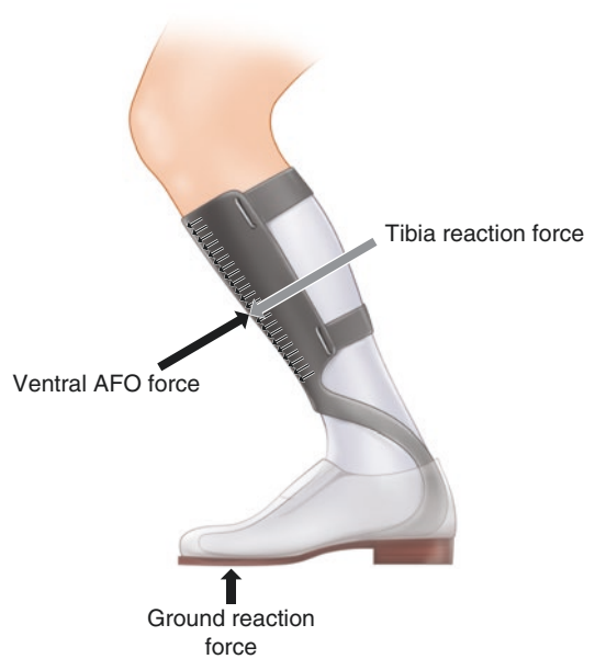
Fig. 14.19 Ankle foot orthosis. In this version, the larger contact area of the ventral AFO allows less pressure placed on the tibia. (Adapted from van der Wilk D, Dijkstra PU, Postema K, Verkerke GJ, Hijmans JM. Effects of ankle foot orthoses on body functions and activities in people with floppy paretic ankle muscles: a systematic review. Clin Biomech (Bristol, Avon). 2015)
