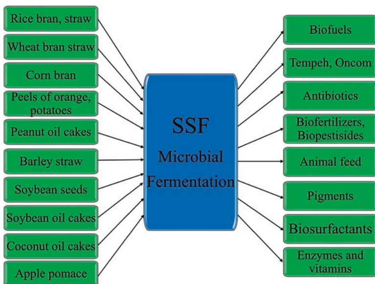
Fig. 1.2 Common agro-industrial wastes and by-products derived through solid state fermentation (SSF). The common agro-industrial wastes such as rice bran and straw, wheat bran and straw, corn bran, peels of orange, peels of potatoes, oil cakes of peanut, soybean, coconut, barley straw, seeds of soybean, apple pomace when subjected to solid-state fermentation can yield beneficial by-products like biofuels, edibles like tempeh and oncom, antibiotics, biofertilizers and biopesticides, nutrient-rich feed for animals, several pigments, biosurfactants, enzymes, and vitamins. (Modified from Sadh et al. 2018)
