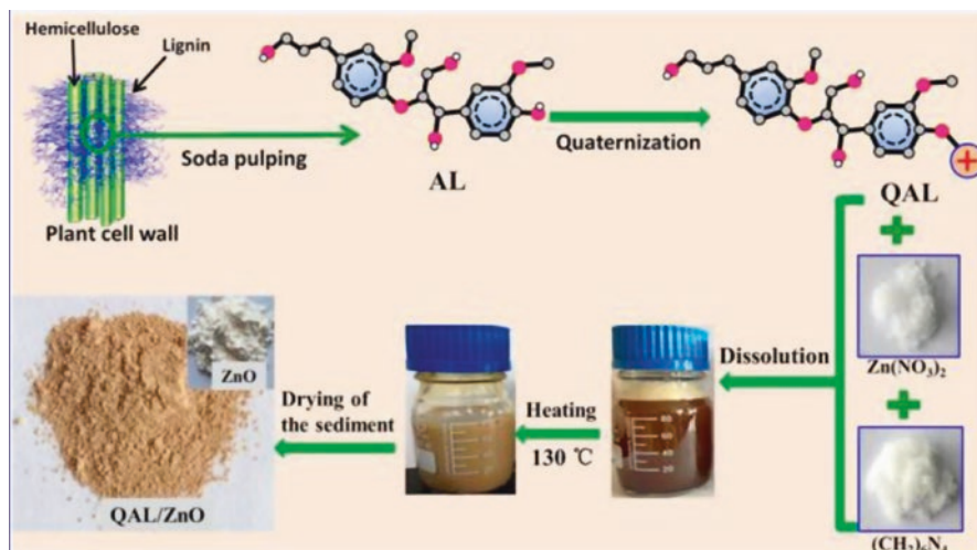
Fig. 4.4 Preparation of quaternized alkali lignin/zinc oxide nanocomposites. (Reprinted with permission from American chemical society (Wang et al. 2017a))
