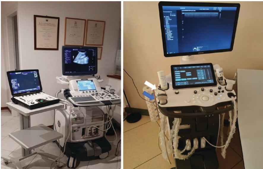
Fig. 8 Portable ultrasound machines with the most common types of transducer probes, linear (white arrow), and convex (blue arrow)
