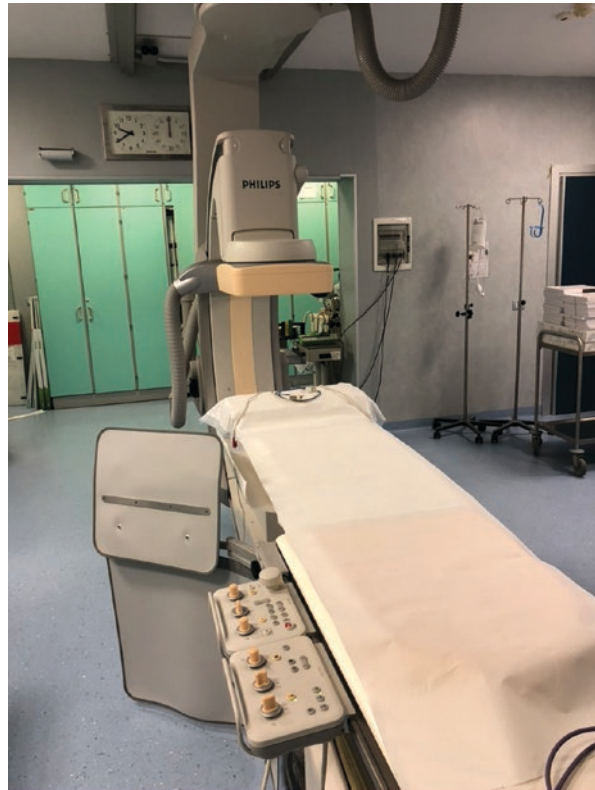
Fig. 3 Standard modern angiographic suite with a C-arm angiography capable of CBCT = cone beam CT, with a spinning fluoro C-arm, and creates CT-like images (with smaller field of view)
