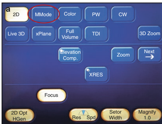
Fig. 5.16 (a) The digital panel indicating the digital button to switch to M-mode imaging (red circle). (b) Parasternal long-axis M-mode imaging of mitral valve
