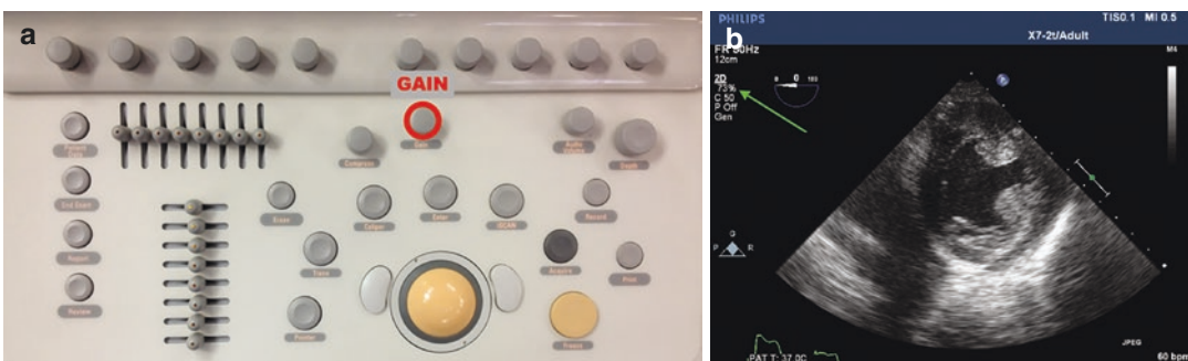
Fig. 5.6 (a) The gain knob on the ultrasound keyboard panel is indicated by the red circle. Turning the knob clockwise increases gain, while turning counterclockwise
