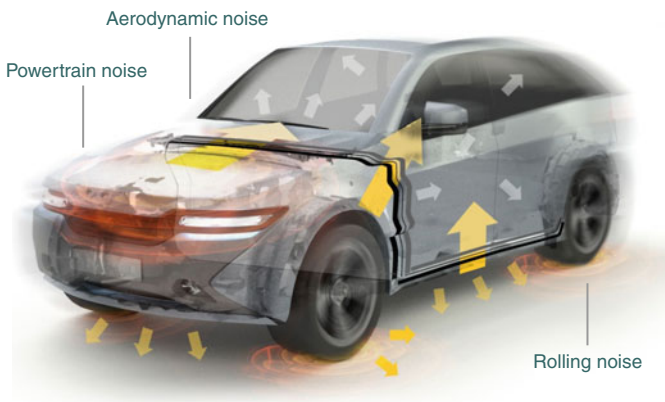
Fig. 11.1 Main sources and transfer paths in a vehicle
