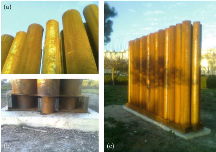
Fig. 3.8 a–c Different views of the sonic crystal acoustic barrier prototype
