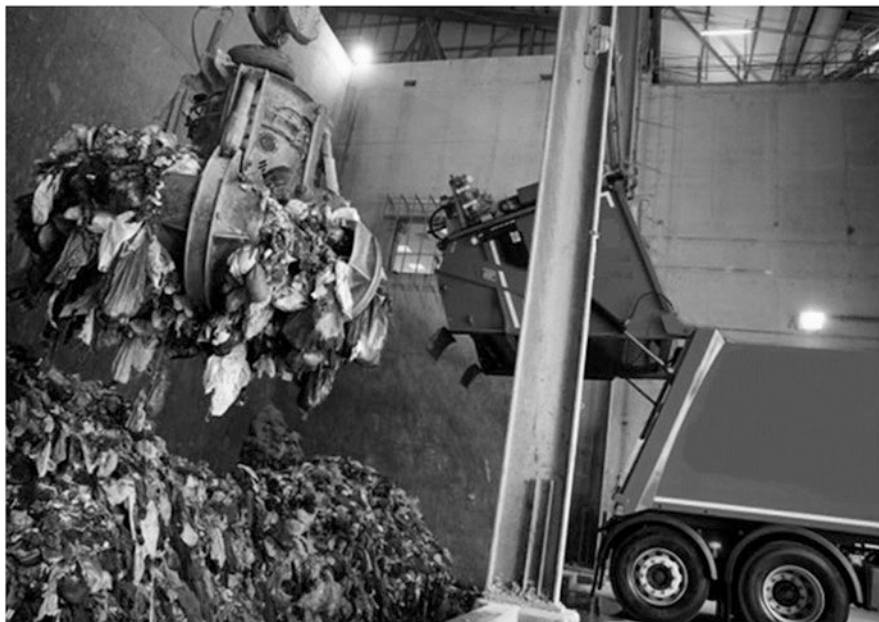
Fig. 3.26 A typical direct discharge station invert [10]
