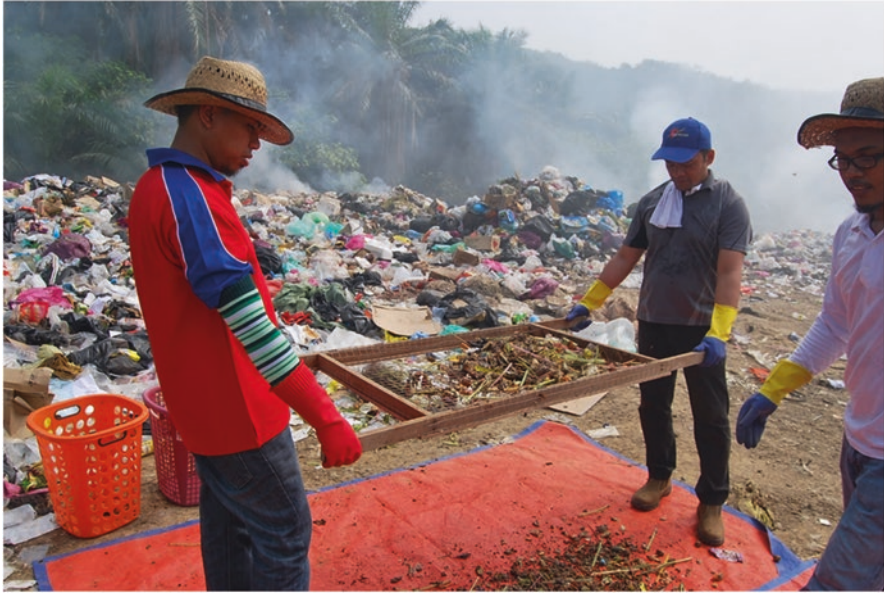
Fig. 4.16 Typical screening process for inert waste
