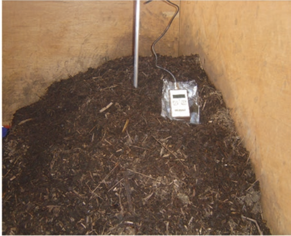
Fig. 7.13 Temperature observation by inserting the thermometer probe into the center of the composting pile [61]
