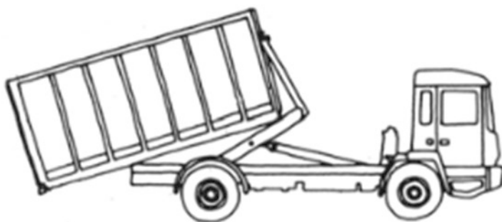
Fig. 3.9 Roll-on–roll-off waste vehicle [30]
