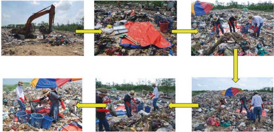
Fig. 4.13 Stepwise of waste composition study based on ASTM
