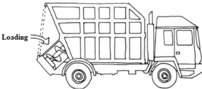
Fig. 3.14 Rear screw compactor vehicle [30]
