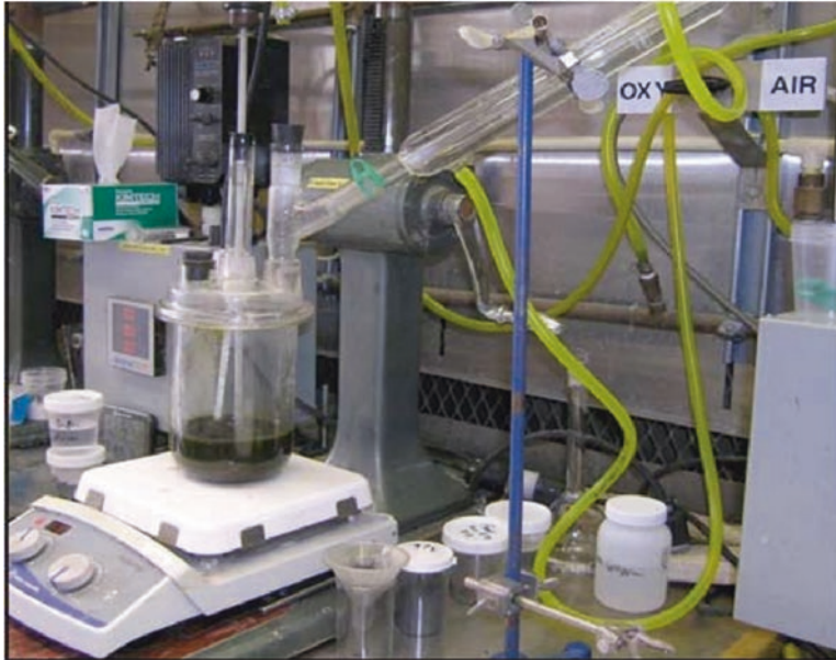
Fig. 4.30 Image of batch leaching test for landfill leachate
