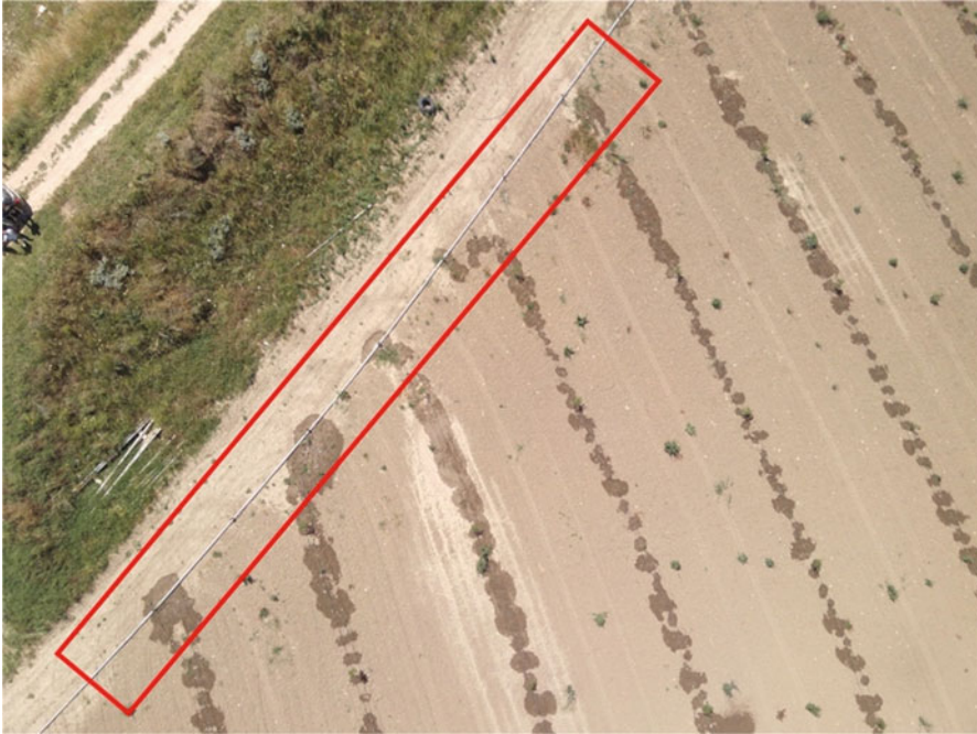
Fig. 11 Testing of a commercial rotary wing UAV in a neophyte orchard for irrigation system monitoring
