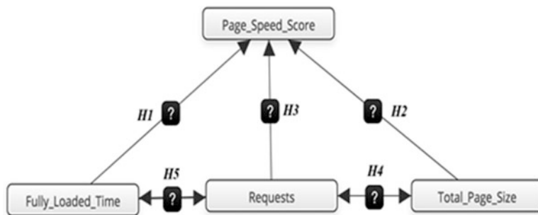
Fig. 2 Fuzzy cognitive representation of possible relationships between the WA metrics via Mental Modeler software as a FCM builder
