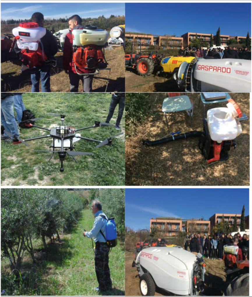
Fig. 5 The various spraying systems used. (Top left: the electrostatic and conventional back pack gas operated blower. Top right: the two commercial electrostatic and conventional large size blower sprayers-2000 L tank. Middle left: the spraying UAV 16 L tank. Middle right: the 16 L tank back-pack electrostatic. Bottom left: the 16 L battery operated back pack and Bottom right: the 1000 L tank conventional mixed spraying system)
