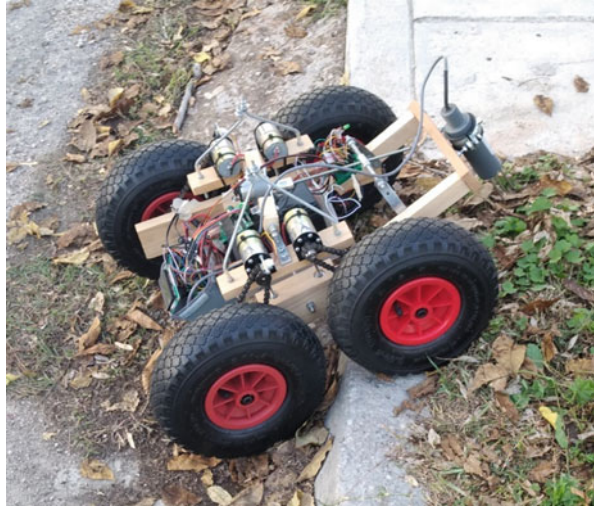
Fig. 9 The flexible chassis layout capabilities of the soil-measurement vehicle allow for graceful obstacle passing
