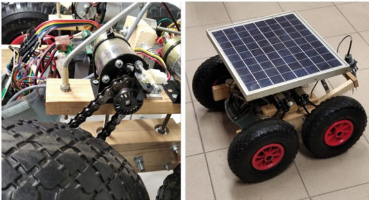
Fig. 5 Details of the photo interrupter sensor disc, attached to the rear wheel sprocket (left), and the solar panel assisted version of the soil measuring robot (right)
