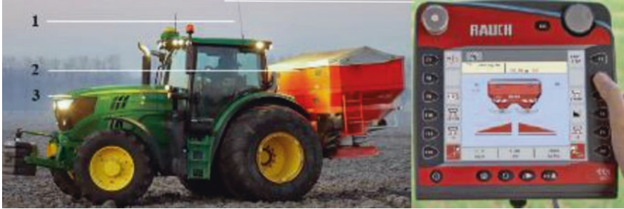
Fig. 34 Variable rate of fertilizer application according to fertilization maps equipment: 1 – Rauchi spreader terminal CCI 100 (Muller); 2 – Mineral fertilizer spreader Rauchi Axis-H; 3 – John Deer 6630 tractor (The figure was prepared by the authors)
