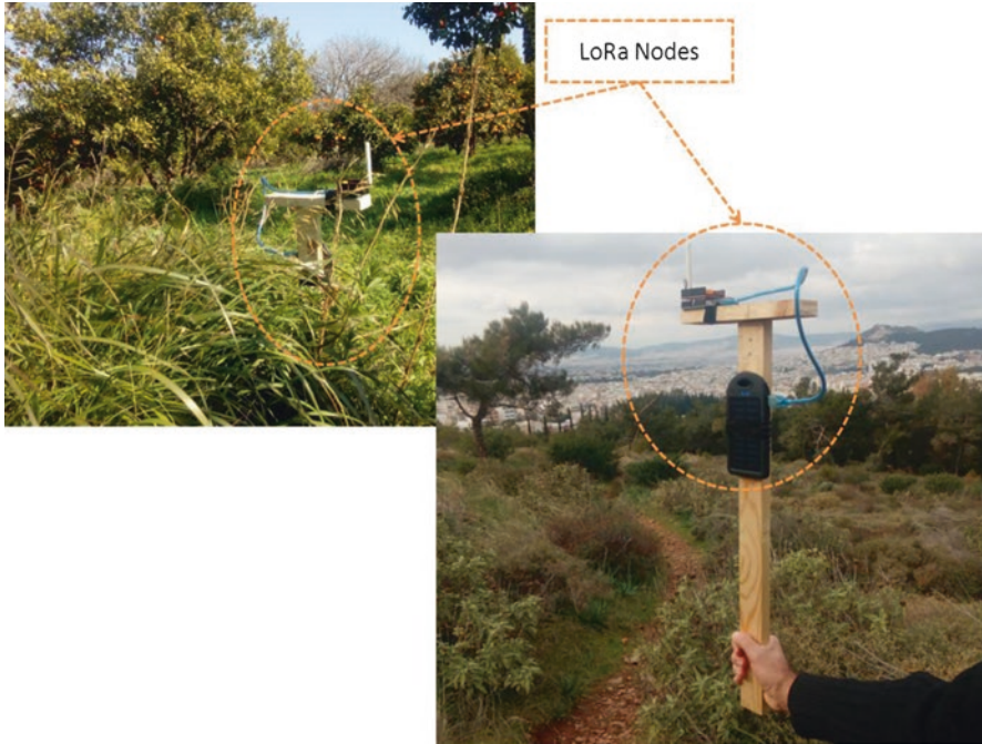
Fig. 6 The experimental measurement equipment, comprising of LoRa modules, in action
