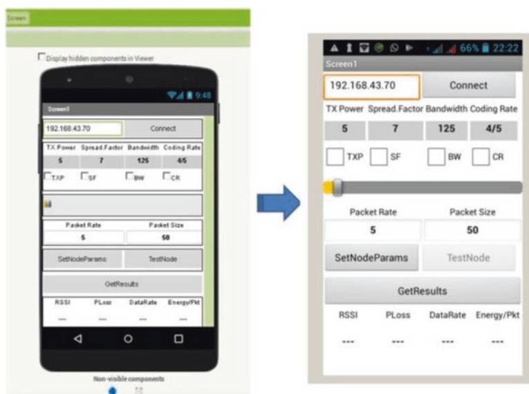
Fig. 2 The main screen layout of the mobile application allowing for a flexible configuration and monitoring of the LoRa nodes
