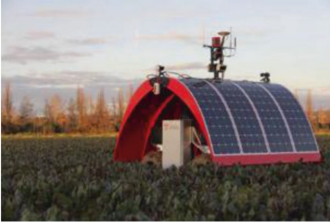
Fig. 16 Solar-powered robot developed in the Australian Center for Fields Robotics, University of Sydney [38]
