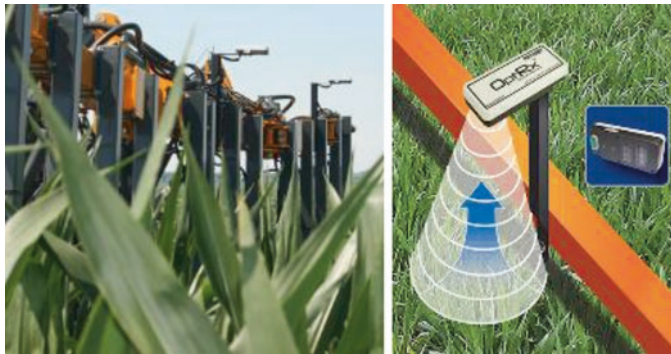
Fig. 13 OptRx crop sensing for real-time variable rate applications [50, 85]
