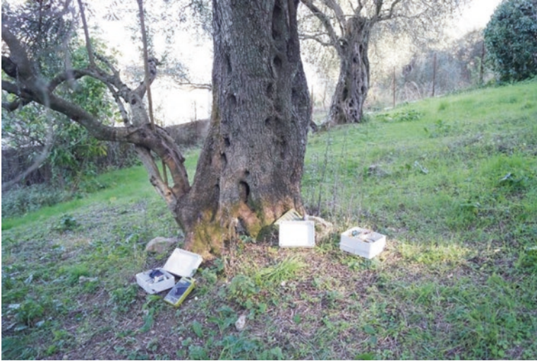
Fig. 4 An installation site on the olive grove, featuring multiple Arduino Uno boards within their protective cases scattered around an olive tree
