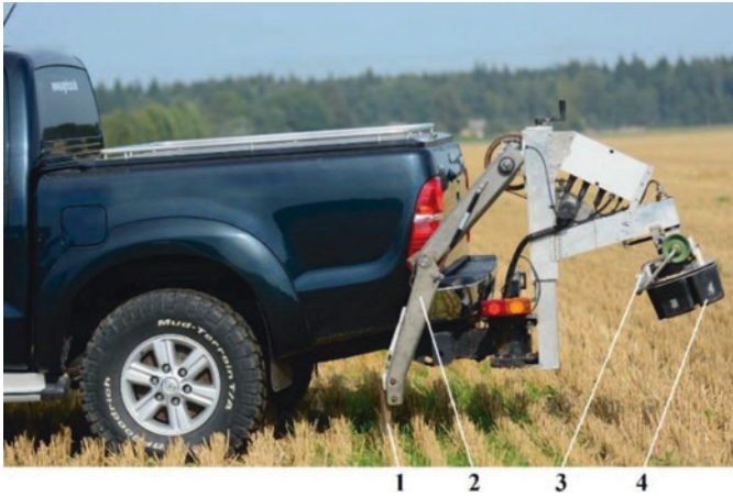
Fig. 32 Automatic soil sampling equipment: 1 – Needle with internal notch for soil sampling; 2 –Automatically operated mechanical hand; 3 – Needle cleaning mechanism; 4 – Box for collecting soil samples (five boxes) (Figure made by the authors)
