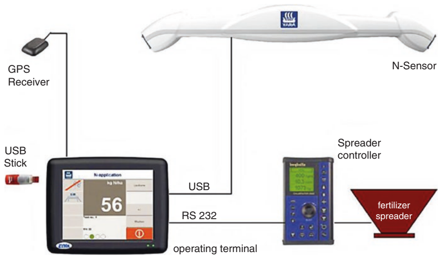
Fig. 12 Schematic of the devices and its connections using Yara N-sensor ALS [84]
