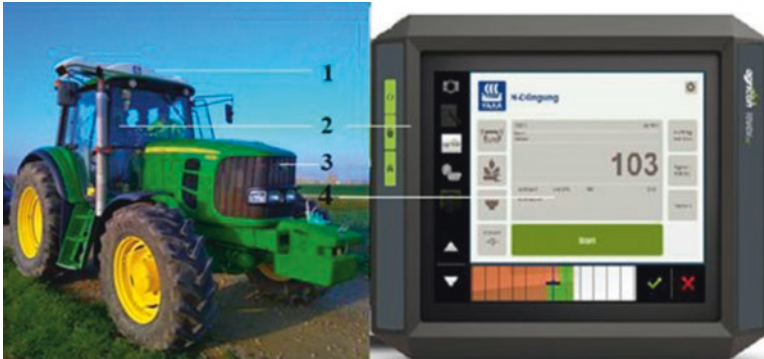
Fig. 40 Equipment used for precision spreading of nitrogen fertilizers: 1 – Yara N-Sensor ALS; 2 – Agricon TOUCH800 terminal (Muller computer); 3 – John Deer 6630 tractor; 4 – Yara N-fertilization software (The figure was prepared by the authors)
