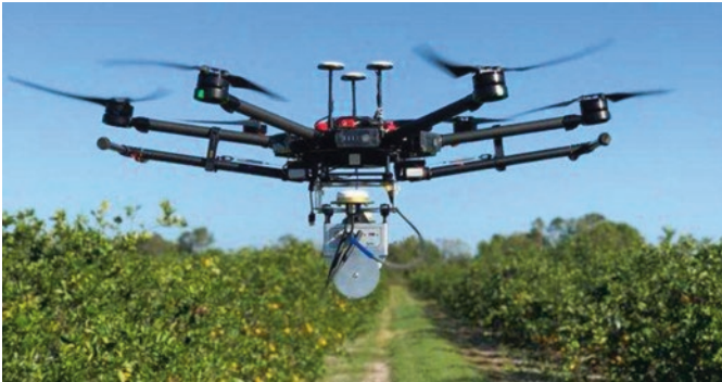
Fig. 7 UAV equipped with a LiDAR airborne sensor
