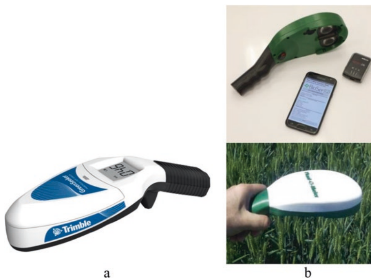
Fig. 3 The two handheld active proximal sensors used in the study; (a) GreenSeeker handheld and (b) Plant-O-Meter
