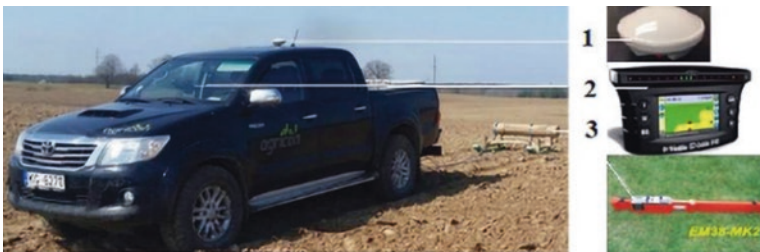
Fig. 29 Mobile determination of field boundaries and soil electrical conductivity: 1 – GPS antenna on the SUV roof; 2 – Trimble EZ-Guide 250 navigation mounted inside the SUV on the windshield; 3 – Electrical conductivity meter EM38-MK2 (Figure made by the authors)
