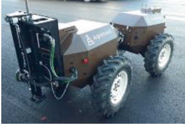
Fig. 15 Universal mobile robot platform for soil sampling [91]
