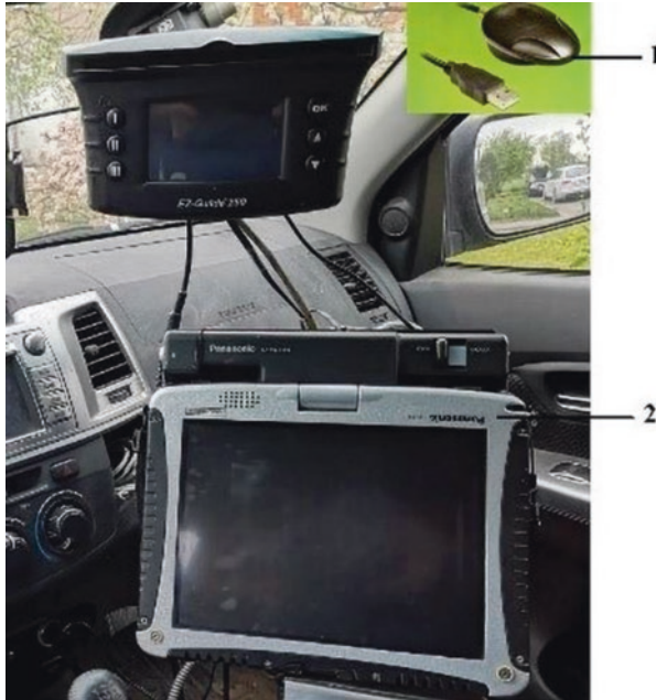
Fig. 30 Data acquisition equipment: 1 – GPS antenna for data collection from EM38-MK2 equipment and recording of sampling trajectories. GPS antenna Navilock 602U for transmission of position and altitude data to Panasonic CF-19 computer; 2 – Panasonic Toughbook CF-19 in the docking station (Figure made by the authors)
