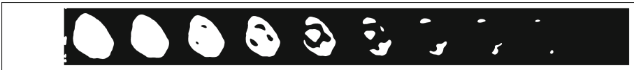
Fig. 4. VGG16: the saliency map for sample ISIC_0000013 thresholded for 0.0 = all-white, 0.1, 0.2, ..., 1.0 = all-black. Corresponding Jaccard indices between ground truth and union feature are 0.064, 0.150, 0.171, 0.189, 0.221, 0.242, 0.243, 0.216, 0.137, 0.059, and 0.000.
