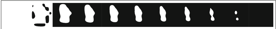
Fig. 5. RESNET50: the saliency map for sample ISIC_0000013 thresholded for 0.0 = all-white, 0.1, 0.2, ..., 1.0 = all-black. Corresponding Jaccard indices between ground truth and union feature are 0.064, 0.104, 0.156, 0.174, 0.174, 0.158, 0.127, 0.101, 0.072, 0.009, and 0.000.
