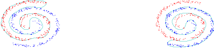
Fig. 2. Negative SVDD applied to a two-spirals shaped data set [20]. It is interesting to note that for changing the target objects it is only necessary to flip the labels. The asterisked points are the SV on the edge, depending on the respective class.
