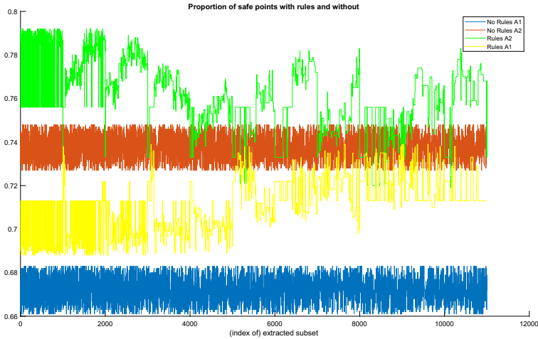
Fig. 6. Using intelligible rules (LLM) the proportion of safe points increases but FNR increases too. (Color figure online)
