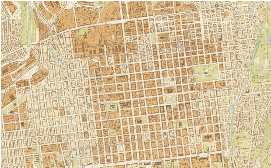
Fig. 2.28 Extract from the Soviet plan of Almaty, Kazakhstan (1967, 1:25,000), distinguishing 'fire-resistant' blocks in orange (National Library of Australia, nla.obj-234565273)
