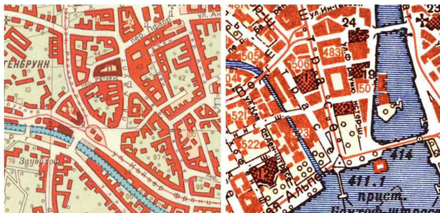
Fig. 2.23 Extract from the Soviet plans of Baden, Austria (1950, 1:10,000) (left) and Zürich, Switzerland (1952, 1:15,000) (right). Given the use of hachuring rather than graduated shades and lack of black building outlines on the plan of Zürich, it has a cruder appearance than the plan of Baden (private collection)
