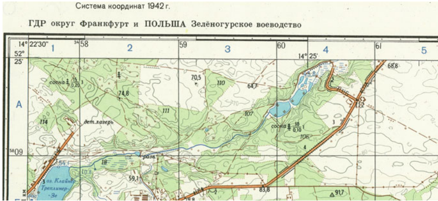
Fig. 2.19 Country and regional information on the Soviet plan of Frankfurt an der Oder, East Germany (1983, 1:10,000). As part of the plan covers Polish territory, 'POLAND Zelenogorsk Voivodeship' is included (private collection)
