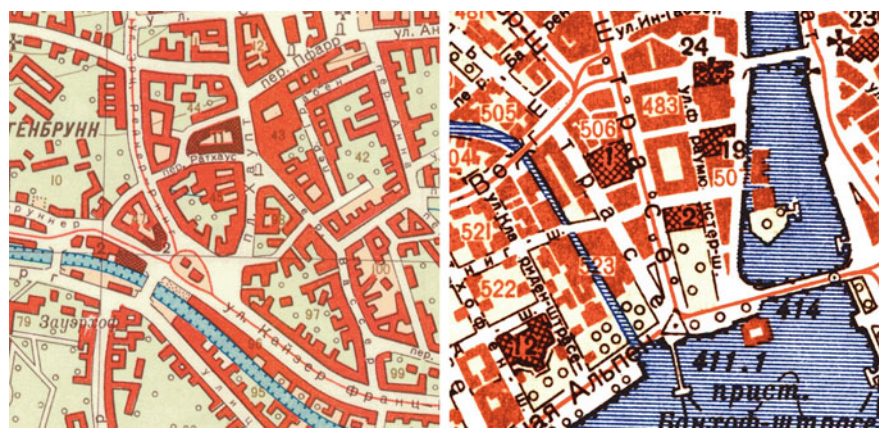
Fig. 2.23 Extract from the Soviet plans of Baden, Austria (1950, 1:10,000) (left) and Zürich, Switzerland (1952, 1:15,000) (right). Given the use of hachuring rather than graduated shades and lack of black building outlines on the plan of Zürich, it has a cruder appearance than the plan of Baden (private collection)
