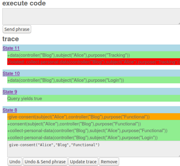
Fig. 4. A web-interface for eFLINT showing (part of) a trace. State 8 is expanded.
