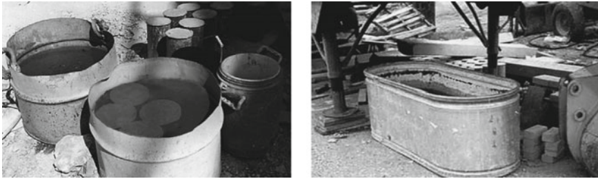
Fig. 3 Water hardening of concrete specimens under construction site conditions
