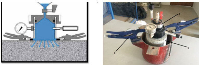
Fig. 2 a) General scheme of the Germann GWT-4000, b) Concrete water penetration rate test. 1-concrete sample, 2-installation GWT-4000, 3-clamps.
