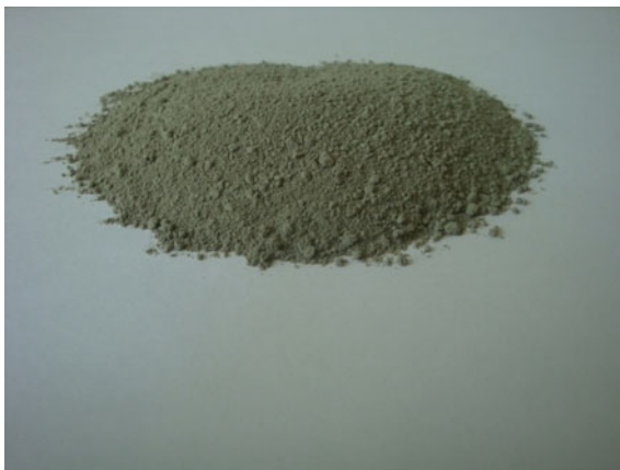
Fig. 2 Electroplating sludge after drying and grinding
