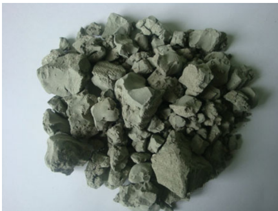
Fig. 1 Electroplating sludge before drying and grinding
