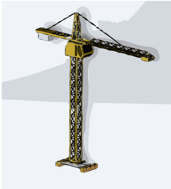
Fig. 1 Tower crane: a—real object; b—full-scale model. Legend: 1—arrow; 2 control cabin; 3—tower; 4—head; 5—cargo trolley; 6—counterweight; 7—thrust
