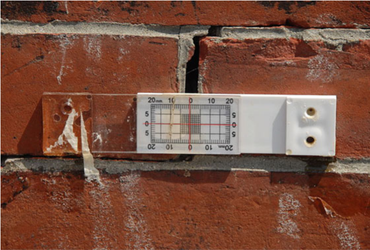
Fig. 6 An example of a visual optical mechanical displacement sensor for the construction tasks, known since the nineteenth century. Application of lensless microscopes with tensoresistive contact elements makes it possible to increase the sensitivity of optical detection by 3–4 orders of magnitude. Open source of the image: Wikimedia
