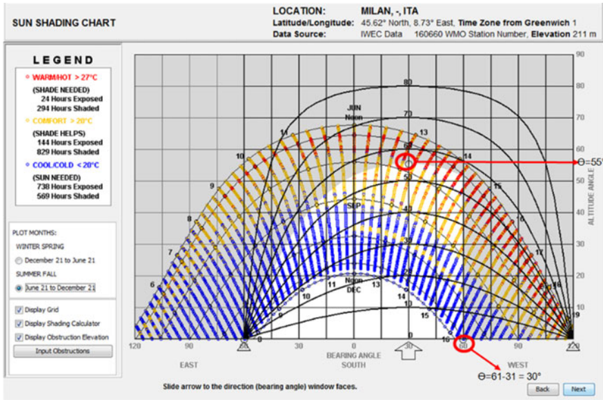
Fig. 6 Sun shading chart for Tunnel façade (south and west-facing façade) shading design
