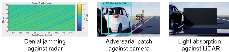
Fig. 8. Examples of sensor attack simulation supported by the prototype
