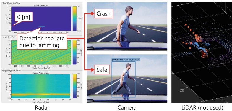
Fig. 11. Evaluation result for detection concatenation. The LiDAR is turned off.
