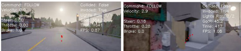
Fig. 1. Sample frame from the videos recorded. Left : the car is driving correctly on the intended lane. Right : an accident caused by the injection of HopSkip Jump. The vehicle does not steer as much as it should, and it goes out of the road, colliding with a building.
