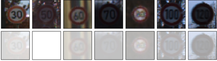
Fig. 5. Counterexamples for model 3A. Upper row is the original image, lower row has perturbation applied at the average level required for misclassification.
