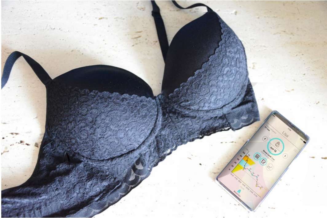
Fig. 7.5 The “Bloomer Bra” features a multi-lead electrocardiogram, accelerometer, and temperature sensor that gather vital information for diagnosticians and deliver real-time, medical-grade data to the user’s smartphone
