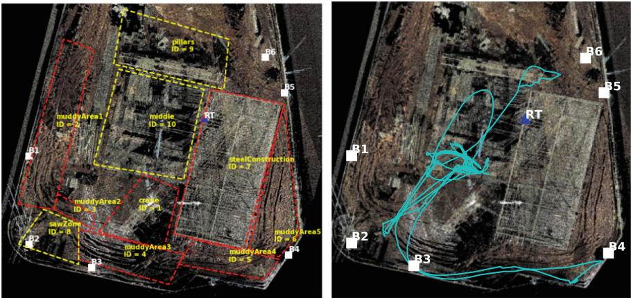
Fig. 2. Left: Semantically meaningful work areas represented as polygons on a construction site. Right: Worker trajectory data (cyan lines) captured via UWB sensors are directly converted into symbolic facts asserting the time intervals during which the worker was located in particular work areas.
