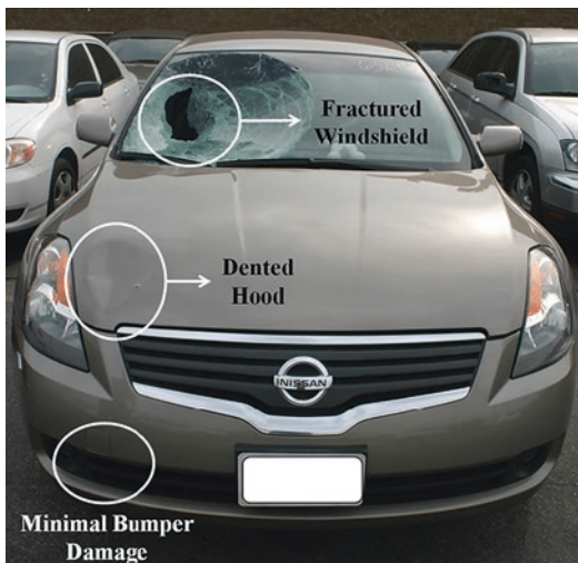
Fig. 21.4 Damage profile to a vehicle that has hit a pedestrian
