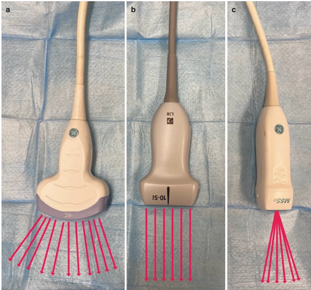
Fig. 26.7 Ultrasound Probes—A: Curved array probe, B: Linear array probe, C: Phased array probe
