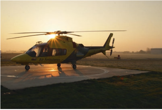
Fig. 19.9 AW109 helicopter. Note the main rotor disk is tilted forwards and so is lower at the nose
