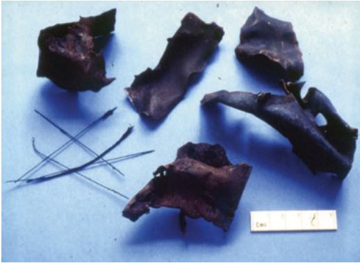
Fig. 38.6 Examples of debris and fragments from IED explosions—typically irregular, larger fragments from casing or object used to disguise the IED
