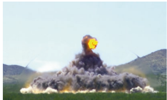
Fig. 38.3 An explosion with the shock wave visible and separating from the rest of the explosion as it travels faster
