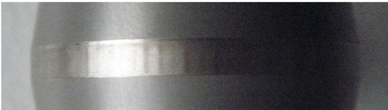
**Fig. 6.** Damaged sample after test without lubricant
