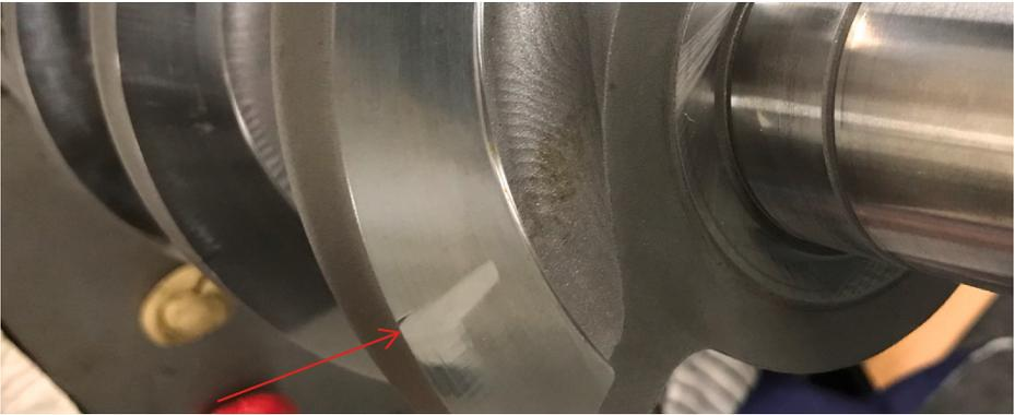
Fig. 9. Axial cam wear after lifetime expectancy tests
