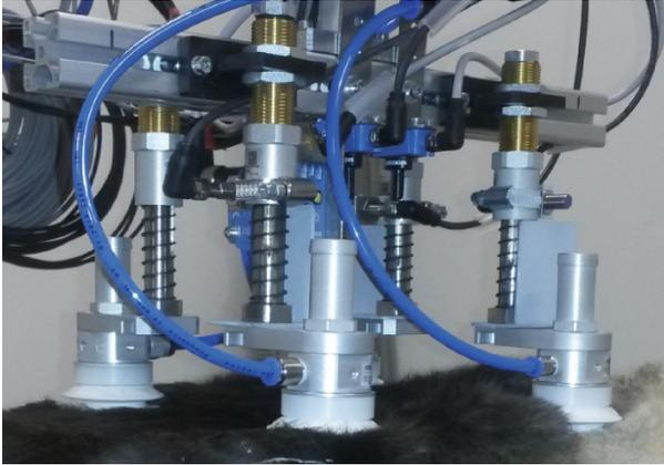
**Fig. 6.** Gripper with ultrasonic sensors for gripping skins
