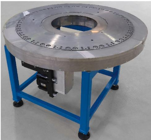
**Fig. 1.** Rotary table assembled
