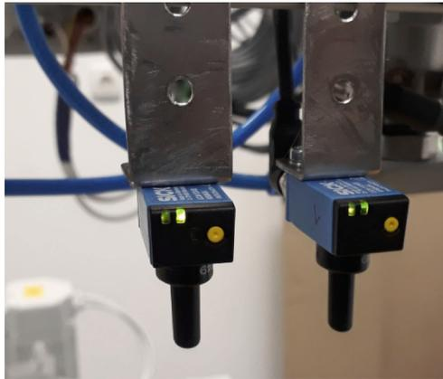
**Fig. 1.** Ultrasonic sensors UC4
