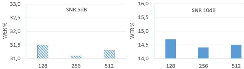
Fig. 5. ASR WER (%) on the TED-LIUM development corpus as function of the size of hidden layer of BERT. SNR of 5 and 10 dB, 4-grams LM, L12Hyyy BERT_{sem} fine-tuned on 1000 talks.
